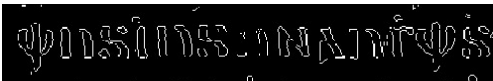
Figure 6.2: The line after being processed by the sobel filter (Matlab)
