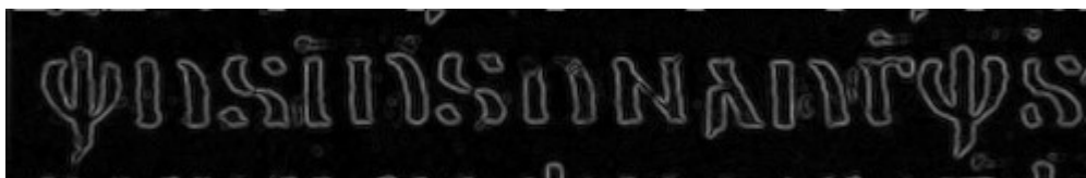
Figure 6.3: The line after being processed by the sobel filter (Gimp)
